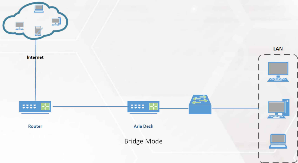
Figure 8- Transparent or Bridge mode of deployment of Ariadezh UTM
